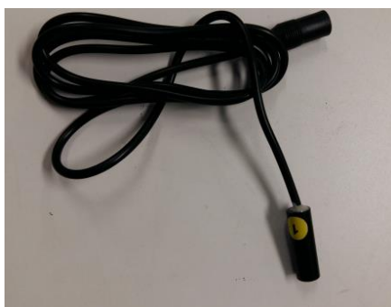
Figure 2: Laser diode with 0.5 mW output at wavelength of 650 nm (Class II)
