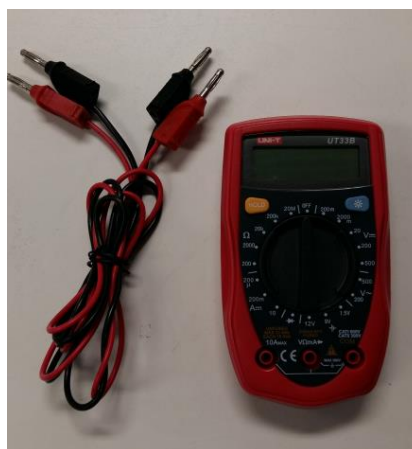
Figure 5: Digital multi-meter and wires with banana connectors
