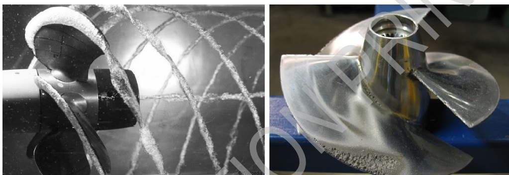
Figure 1. (a) Cavitating propeller (b) Cavitation damage (Source: Wikimedia Commons)
