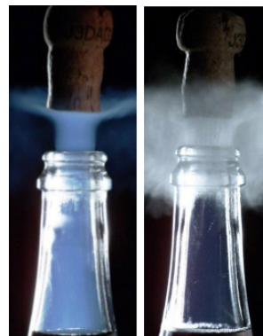
Fig. 6. Left: traditional bottleneck: (1) surrounding air, (2) cork stopper, (3) headspace, (4) liquid champagne. Right: Two phenomena observed while opening the bottle at two different temperatures (adapted from [2]).
