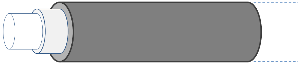
Figure 1.4 Diagram of a fiber optic cable.
